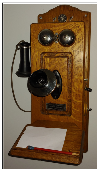
This is an example of an oak wall-mounted crank telephone from the early 1900s. The tag on the front reads “Chicago Telephone Supply Company, Elkhart, Indiana, U.S.A.”
